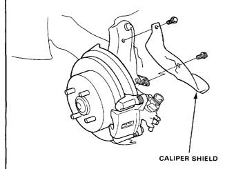
Remove the two caliper mounting bolts and the caliper from the bracket.
