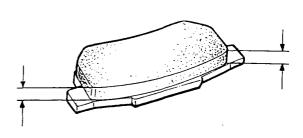
If the lining thickness is less than service limit, replace the brake pads as a set.
