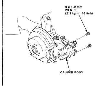
4. Remove the pads and measure the thickness of each brake pad lining using a vernier caliper.
