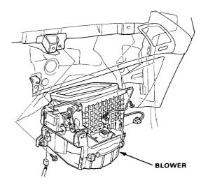
Install the blower in the reverse order of removal and make sure there is no air leakage.
