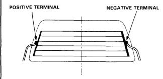
2. Check for continuity between the negative terminal and body ground.
