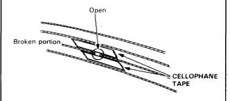
Using a small brush, apply heavy coat of silver conductive paint extending about 1/8 in. on both sides of the break. Allow 30 minutes to dry.
