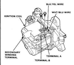
Using an ohmmeter, measure resistance between the terminals. Replace the coil if the resistance is not within specifications.
