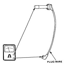
If resistance exceeds 25,000 ohms, replace the ignition wire.
