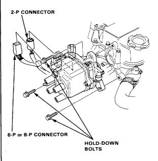
Remove the distributor hold-down bolts, then remove the distributor from the cylinder head.
