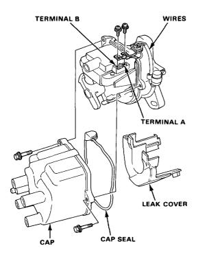
3. Remove the 4 screws and slide the ignition coil out of the distributor housing.
