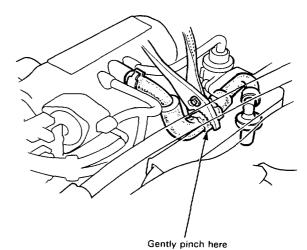
If there is no clicking sound, check the PCV valve grommet for cracks or damage. If the grommet is OK, replace the PCV valve and recheck.
