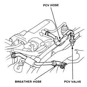
At idling, make sure there is a clicking sound from the PCV valve when the hose between PCV valve and intake manifold in lightly pinched with your fingers or pliers.
