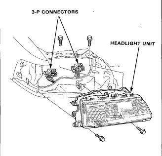
After installing the unit, adjust the headlights to local requirements.
