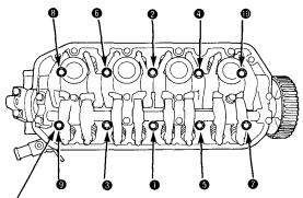
CYLINDER HEAD BOLT 10 x 1.25 mm 68 N·m (6.8 kg·m, 49 lb-ft)
