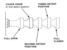
Fast idle should be: 1,500-2,500 min<sup>-1</sup> (rpm)
