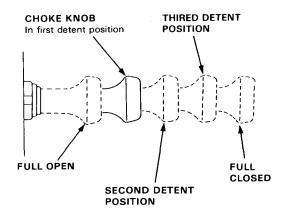
Fast idle should be: 1,500-2,500 min<sup>-1</sup> (rpm)
