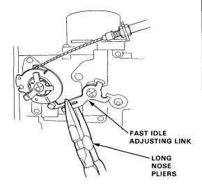
If the engine speed is too low, insert a screwdriver in the fast idle adjusting link slot and widen the slot.
