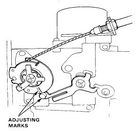
If not aligned, loosen the locknut and adjust the adjusting nut, then retighten the locknut.
