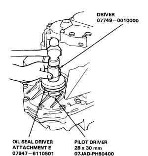
2. Install the oil seal in the torque converter housing.
