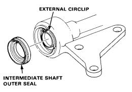
3. Remove the intermediate shaft.
