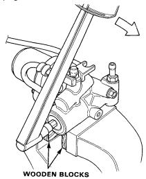
NOTE: Clamp the pump in a vise only as shown adove.
