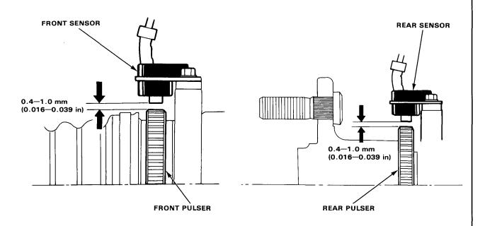
Measure air gap between the sensor and pulser all the way around while rotating the driveshaft by hand.
