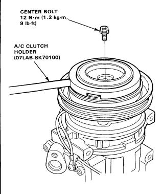
2. Remove the pressure plate and shim(s) taking care not to lose the shims.
