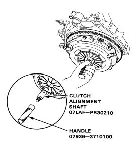
Torque the bolts in a crisscross pattern as shown. Tighten them two turns at a time to prevent warping the diaphragm spring.
