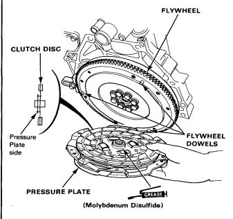
4. Install the attaching bolts finger tight.
