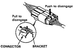
When disconnecting locks, first press in the connector tightly (to provide clearance to the locking device), then operate the tab fully and remove the connector in the designated manner.
