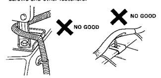
Route harnesses so they are not pulled taut or slackened excessively.
