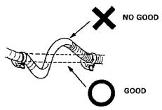
Protect wires and harnesses with a tape or a tube if they are in contact with a sharp edge or corner.
