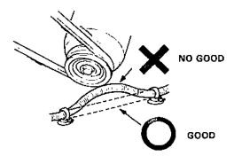
Always keep a safe distance between wire harnesses and any heated parts.
