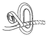
Clean the attaching surface thoroughly if an adhesive is used. First, wipe with solvent or alcohol if necessary.
