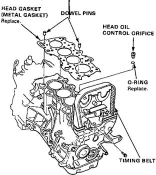
Tighten cylinder head bolts in two steps. In the first step tighten all bolts, in sequence, to about 30 N·m (3.0 kg-m, 22 lb-ft); in the final step tighten, in same sequence, to 85 N·m (8.5 kg-m, 61 lb-ft) NOTE: Apply engine oil to the cylinder head bolts and the washers.
