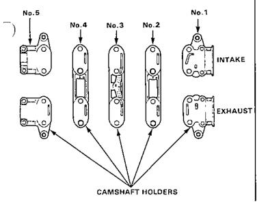
Set the camshaft folders and camshaft holder pipes, then tighten temporaly the bolts.
