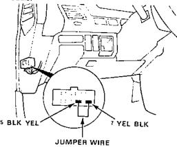
Check that battery voltage is available at the fuel pump connector when the ignition switch is turned ON (positive probe to the YEL/BLK wire, negative probe to the BLK wire).
