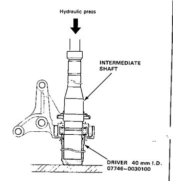
Seat the 38 mm external circlip in the groove of the intermediate shaft.
