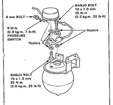
3. Remove the accumilator nut as shown.
