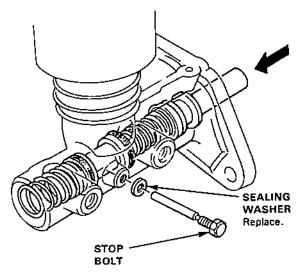
Remove the piston guide, secondary piston assembly and pimary piston assembly.
