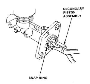
Remove the stop bolt while pushing in the secondary piston assembly.
