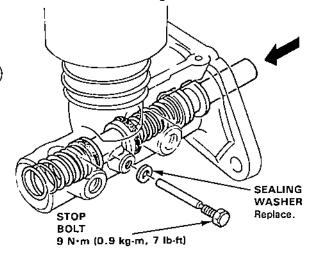
Press the secondary piston in and install the new snap ring.
