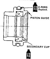
Make sure that the primary piston assembly and secondary piston assembly are in good condition.
