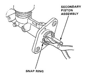
CAUTION: Avoid damaging the sliding surface of the secondary piston when installing the sanp ring.
