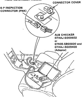
NOTE: The adaptor 07HAJ-SG00400 is not necessary when using of the checker 07HAJ-SG00602.
