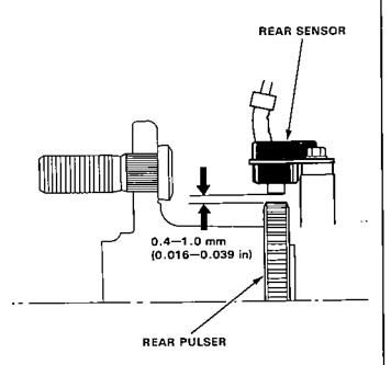
Measure air gap between the sensor and pulser all the way around while rotating the driveshaft by hand.
