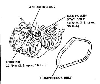
Remove the compressor mounting bolts (4) and compressor. Rest the compressor on the front beam.
