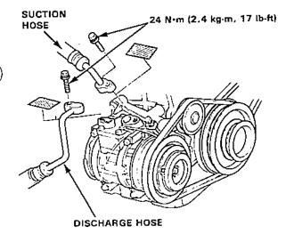
Disconnect the compressor connector and the clamp.
