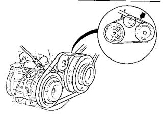
②When using ND tension gauge;
