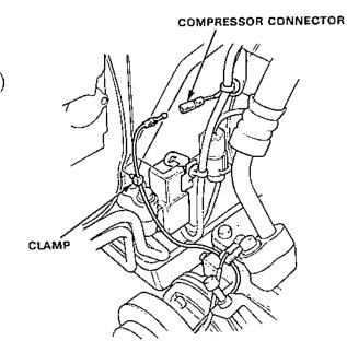
Loosen the idle pulley stay bolt. Loosen the lock nut and adjusting bolt, then remove the compressor belt.
