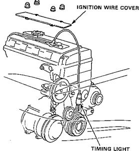
Adjust ignition timing, if necessary, to the following specifications:
