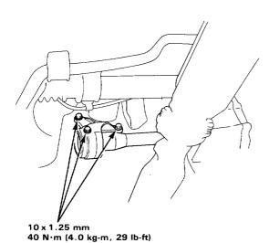
Lower the bearing support close to the steering gearbox and remove the intermediate shaft from the differential.
