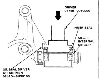
4. Press the intermediate shaft into the shaft bearing.
