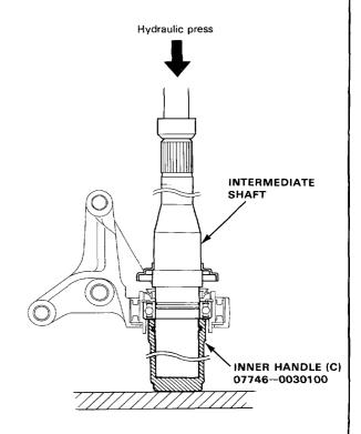
Seat the 38 mm external circlip in the groove of the intermediate shaft.
