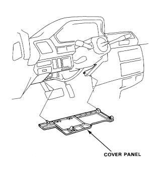
5. Remove the steering joint cover.
