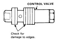
Slip the valve back in the pump and check that it moves in and out smoothly.
