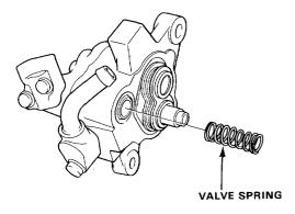
4. Check for wear, burrs, and other damage to the edges of the grooves in the valve.
