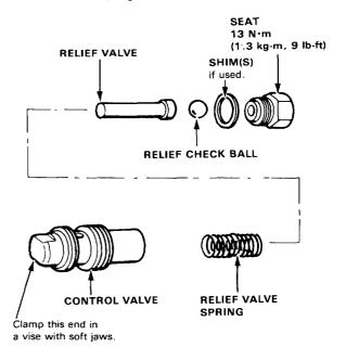
Clean all the parts in solvent, dry them off, then reassemble and re-test the valve.
