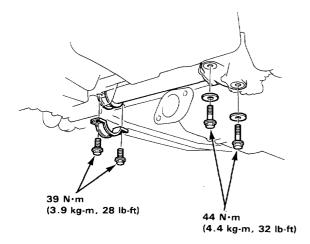
18. Slide the gearbox right so that the left tie rod clears the bottom of the rear beam, then remove the gearbox.
