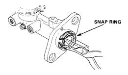
5. Install a new rod seal.
