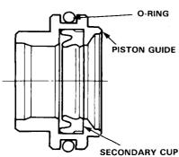
2. Install the piston assemblies in the master cylinder.
