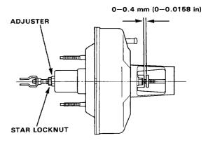
NOTE: If the clearance between the gauge body and adjusting nut is 0 mm, the push rod-to-piston clearance is 0.04 mm. If the clearance between the gauge body and adjusting nut is 0.4 mm, the push rod-to-piston clearance is 0 mm.
