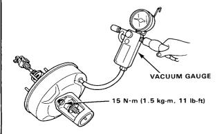
• Inspection with the booster attached to the car.
