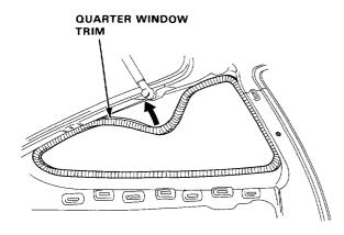
With a sponge, apply a light coat of body primer to the original adhesive remaining around the window opening flange.
