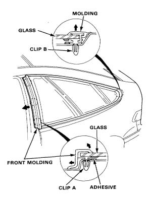
Remove the quarter glass molding if the glass is to be reused.
