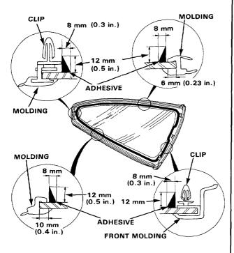
12. Use suction cups to hold the glass, then set it on the adhesive. Lightly push on the glass until its edges are fully seated on the adhesive all the way around.
