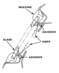
As an assembly, pry the glass and upper and front moldings away from the car at the clip points shown.
