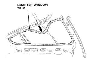
From inside the car, use a knife to cut through the glass adhesive all the way around.
