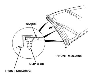
Install the quarter molding on the glass by using the clips shown.
