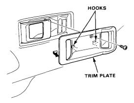
Remove the power window switch, if equipped, from the trim plate by removing the 4 screws.
