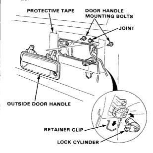
Pull the outside door handle out, and pry the joint off the handle with a flat-tip screwdriver. Remove the handle from the rod. Remove the screws, take the door latch off the door, then push the door latch and rod inside the door.
