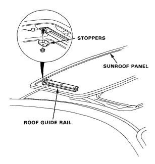
Remove the front mounting bolts. Remove the sunroof panel from the rear slide bracket by sliding it forward by hand.
