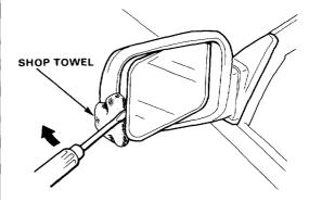
Install the mirror in the reverse order of removal, and also apply grease to the location shown.
