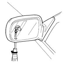
2. Carefully pry out the mirror with a flat-tip screwdriver as shown.
