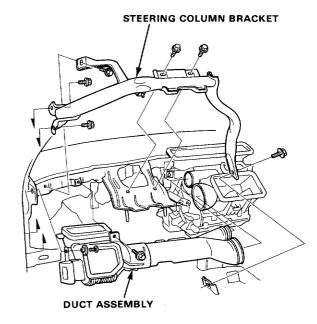
Remove the heater mounting bolts (2), disconnect the wire harness connector from the function control motor, and then remove the heater assembly.
