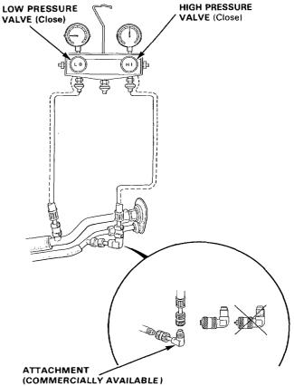
NOTE: Set the attachment to the gauge hose at high pressure side first, then install the gauge set as shown. When disconnecting the gauge hose at high pressure side, remove the attachment from the high pressure charging valve.
