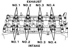
Set the No. 1 piston at TDC. "UP" marks in the pulleys should be at top, and the TDC grooves on back side of pulley should align with cylinder head surface. The distributor rotor must be pointing towards No. 1 plug wire.
