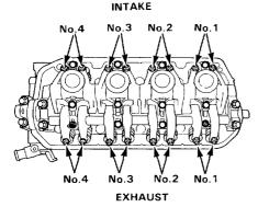
Set No. 1 piston at TDC. "UP" mark on the pulley should be at top, and TDC grooves on the pulley should align with cylinder head surface. The distributor rotor must be pointing towards No. 1 plug wire.
