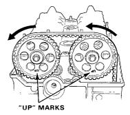
Rotate crankshaft 180° counterclockwise to bring No. 2 piston to TDC. "UP" marks should be at intake side. Distributor rotor should point to No.2 plug wire. Adjust valves on No.2 cylinder.
