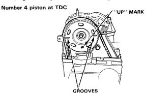
Rotate crankshaft 180° counterclockwise to bring No. 2 piston to TDC. The "UP" mark should be at intake side. Distributor rotor should point to No. 2 plug wire. Adjust valves on No. 2 cylinder.
