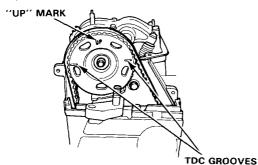
3. Adjust valves on No.1 cylinder. Intake: 0.17-0.22 mm (0.007-0.009 in.)
