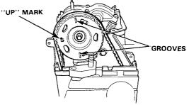
Rotate crankshaft 180° counterclockwise to bring No. 4 piston to TDC. Both TDC grooves are once again visible and distributor rotor points to No.4 plug wire. Adjust valves on No.4 cylinder.
