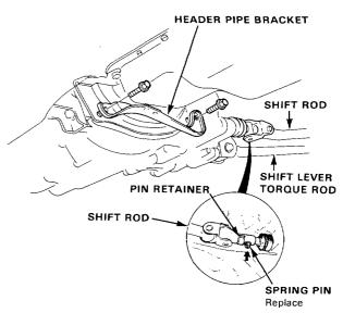
NOTE: On reassembly, slide the retainer back into place after driving in the spring pin.
