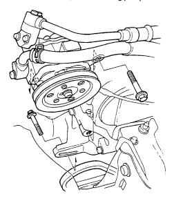
Disconnect the suction and discharge hoses from the compressor.
