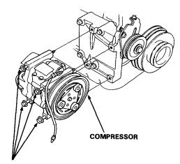
COMPRESSOR MOUNTING BOLTS 25 N·m (2.5 kg-m, 18 lb-ft)
