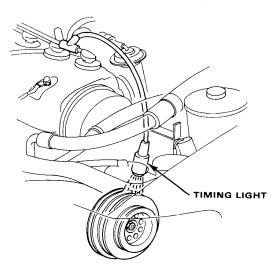
While the engine idles, point the light toward the pointer on the timing belt cover.
