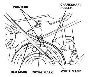
Read initial timing when initial timing mark is aligned to the pointer.
