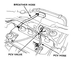
Remove the PCV valve from the intake mainfold and connect a vacuum pump.
