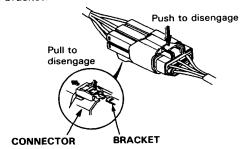
When disconnecting locks, first press in the connector tightly (to provide clearance to the locking device), then operate the tab fully and remove the connector in the designated manner.
