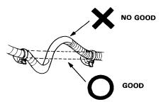
Protect wires and harnesses with a tape or a tube if they are in contact with a sharp edge or corner.
