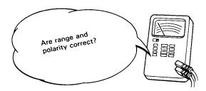
Always insert the probe of the tester from the wire harness side (except waterproof connector).
