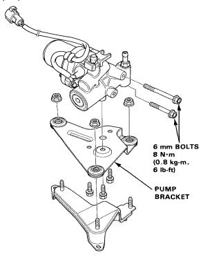
Separate the motor from the pump while rotaing the pump right and left.
