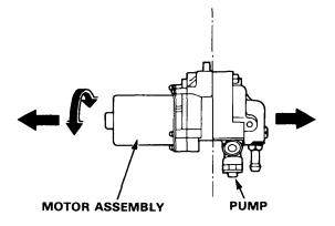
NOTE: About 10 cc(0.6cu-in)of brake fluid will flow out when the motor is removed from the pump.
