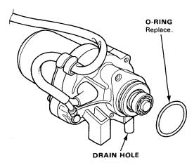
NOTE: Do not wash or dip the motor in brake fluid. Also be careful not to allow oil or water to enter the inside through the water drain hole.
