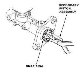
Remove the stop bolt while pushing in the secondary piston assembly.
