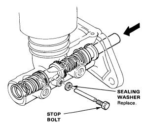
Remove the piston guide, secondary piston assembly and pimary piston assembly.
