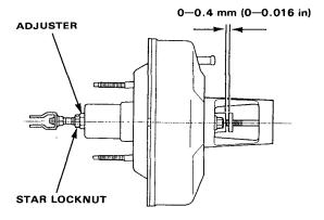
NOTE: If the clearance between the gauge body and adjusting nut is 0 mm, the pushrod-to-piston clearance is 0.4 mm. If the clearance between the gauge body and adjusting nut is 0.4 mm, the pushrod-to-piston clearance is 0 mm.
