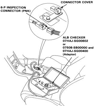
NOTE: The adaptor 07HAJ-SG00400 is not necessary when using of the checker 07HAJ-SG00602.
