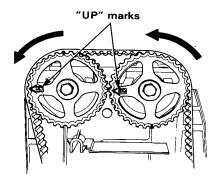
Rotate the crankshaft 180° counterclockwise to bring No.4 piston to TDC. Both TDC grooves are once again visible. Adjust valves on No.4 cylinder.
