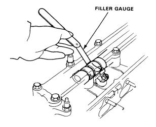
Rotate the crankshaft 180° counterclockwise (campulley turns 90°). The "UP" mark should be on the exhaust side. Adjust valve on No.3 cylinder.
